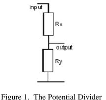
where Rx + Ry is the total value of the equivalent potentiometer, Ry is the sum of all the resistors in the chain to give the attenuation at a given point and Rx is the remainder of the resistor chain. What we actually want to calculate is the value of each individual resistor in the chain to give us the range of attenuations required. Rearranging the above equation, we get:
